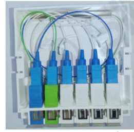
1x4 High Loss Splitter 1:5 Unevenly divided
